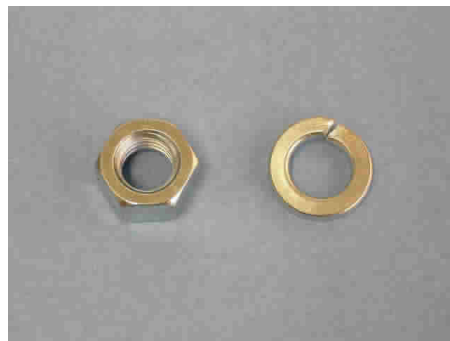
34149 Hex Nut 1/2-13 Zinc * 32455 Lock Washer 1/2" Zinc * Torque to 30-40 ft. lbs.
